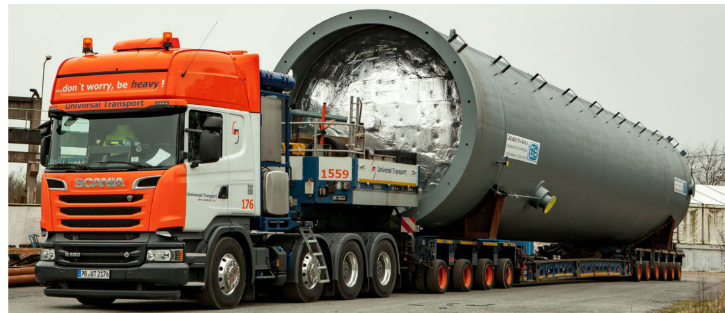
Above: The insulating containers which will be used to store liquid as well as gas are 26,70 m long, 4,90 m wide, 4,58 m high and weigh in at 60 tons each
