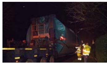
in Germany permit loads measuring more than 5.2 metres. After several months of preparation, it was finally time. A total of five vehicles, each just under 35 metres long, 5.2 metres wide and almost 5.4 metres high headed from Denmark to North Frisia, 200 kilometres away. En route, numerous measures had to be taken to ensure safe passage, such as turning traffic lights out of the way and lifting telephone lines.
