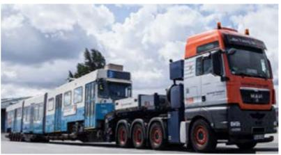
These trailers enable Universal Transport to load and unload cargo completely independently autonomously without crane or forklift truck assistance. Thanks to the investments into our fleet, moreover, it is possible to easily adjust to different track gauges such as the European narrow and standard gauges, the Russian wide
