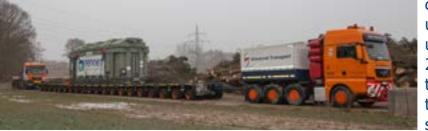
consisting of a push-pull truck unit with two four-axle tractor units and one trailer each with 20 modular axles, started on their way on time at 10:00 p.m. to head to the Ohlensehlen substation near Kuppendorf. The
