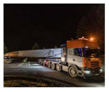
In two consecutive nights, a total of 12 transports, each with a length of 52 metres and a total weight of approx. 130 tonnes per transport, were carried out for a customer in Eichenzell in the Fulda district. The cargo was concrete beams, more precisely prefabricated beams, which are usually made of reinforced concrete and are needed for the construction of a hall in the surrounding area.
